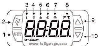
Figura 6: Controlador Digital MT 444E FASTON
