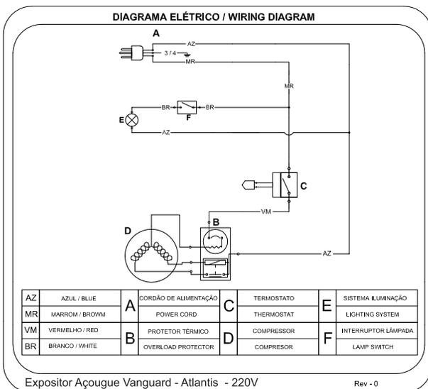
DIAGRAMA ELÉTRICO / WIRING DIAGRAM
